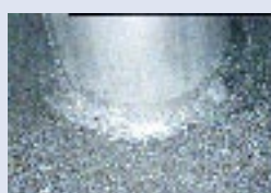
Pickled weld on a 4404 specimen. Please note that the specimen appears slightly mat – almost like after a glass blasting. This is because of the increased surface roughness due to the etching of the steel.
